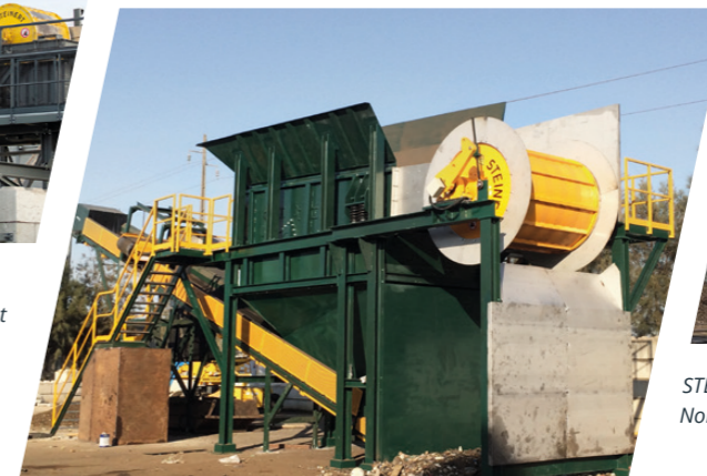
STEINERT MTE Q removes residues and non-ferrous materials in a recycling plant in Spain
