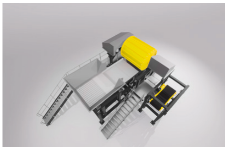
Layout 1: Set up with vibration feeder and STEINERT MTE plus STEINERT UME on STEINERT MTE drop material stream.
