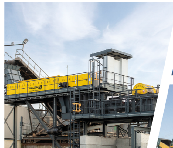
STEINERT SteelMaster installation under way in an end-of-life vehicle recycling plant in Belgium
